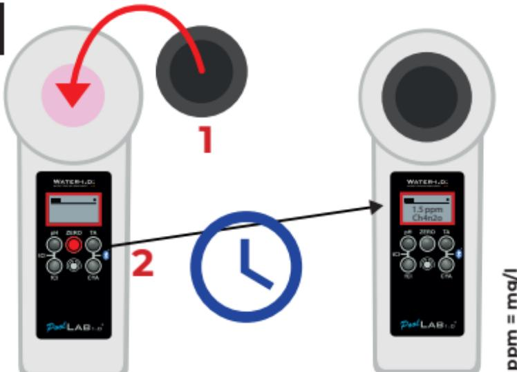
If the sample contains free chlorine, a „Dechlor“ tablet has to be added to the vial, before adding PL Urea 1 and PL Urea 2. Ammonia N°1 only dissolves entirely after Ammonia N°2 was added. Ammonia and chloramines will be detected together. The result displayed will show the sum of both.
