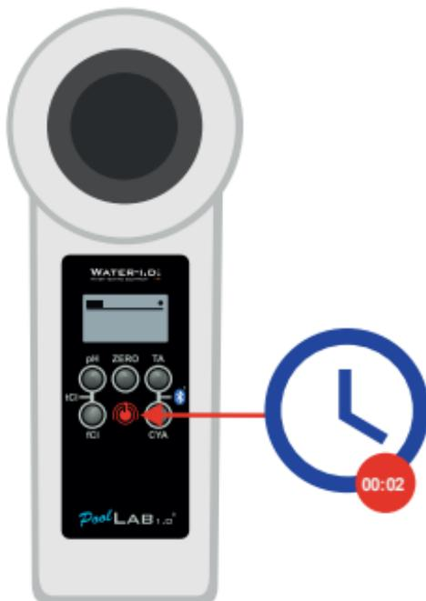
The On/Off button can also be used to skip countdown during measurement (not recommended).
