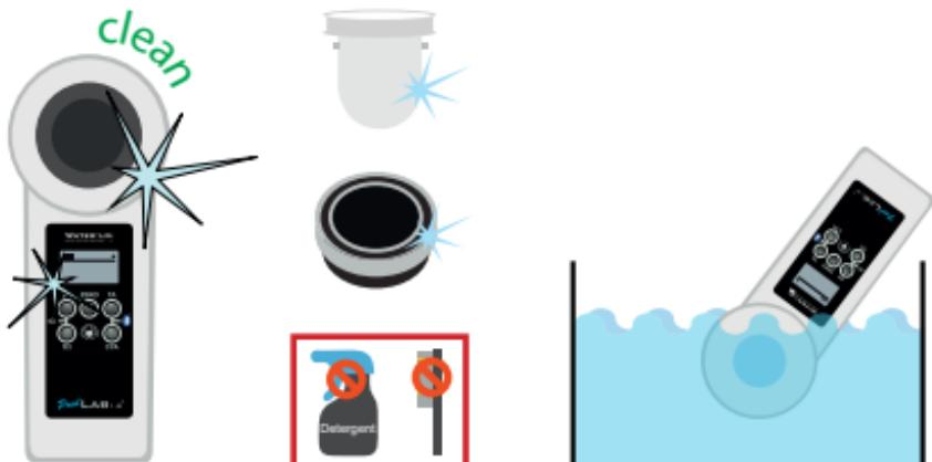
It is important to clean the device after each measurement to get rid of any reagent residues! Please ensure that the cuvette has been cleaned before each measurement (e.g. under clear water/or simply rinsing the cuvette in the pool is sufficient as long as no residues remain).
